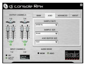
In ASIO mode, you can adjust the following settings: Sample Rate, Sample Size, ASIO Buffer Size.
