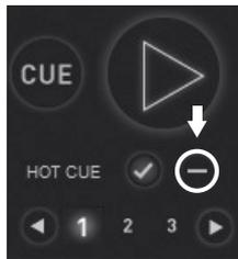
On the DJConsole RMX2: in Hot Cue mode, press the **SHIFT** button and then press one of the pads corresponding to the Cue point that you want to delete.
