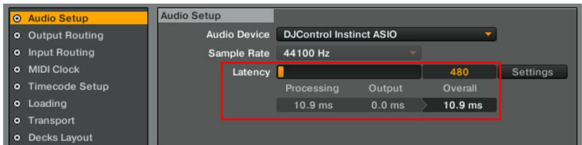
Notice that the parameter **Latency** reflects the value selected in the control panel. This is always a good sign that the application is communicating with the driver properly.
