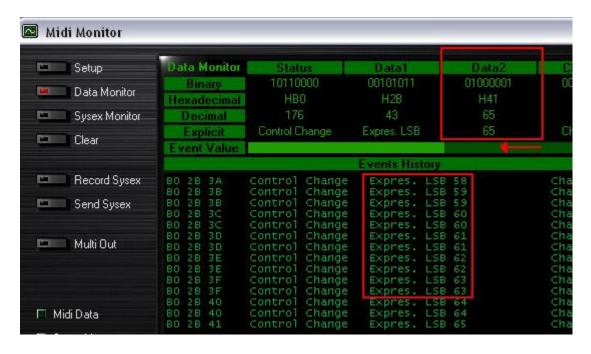
This test can also help determine if some of the controls of the DJ Control are not working correctly. For example, if the crossfader is only halfway to his course but already displays its maximum value of 127.
