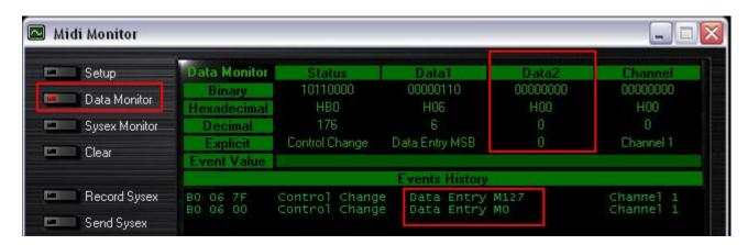
For incremental controls, such as knobs and sliders, you should normally get values **between 0 and 127**, depending on the position of the controller. The **Event Value** should also display the relative position of the control being used according to the value.
