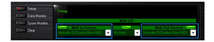
By default, the **MIDI In Device** should be **Open**. This is necessary for the software to be able to read the incoming data from the controller.
