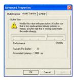
The **Audio Transfer** tab deals with software monitoring. It allows you to configure the monitoring quality by regulating the number of packets per buffer. The fewer the packets, the more the latency is reduced, although some configurations may become unstable as a result. Conversely, a buffer made up of a greater number of packets increases the latency time but helps to ensure system stability.
