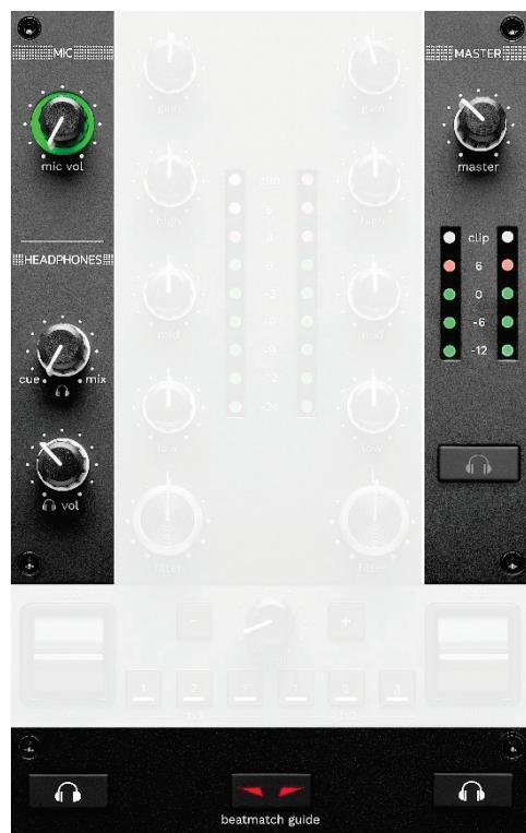
**MIC volume:** adjusts the volume of the microphone.
