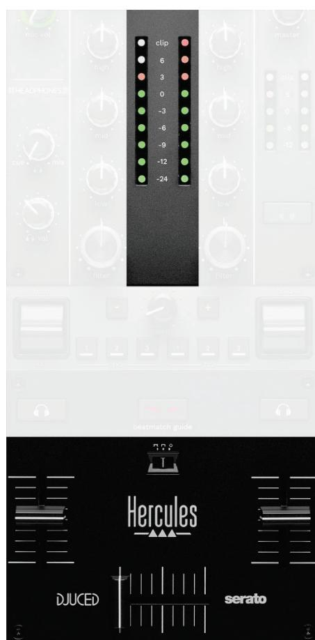
**VU meter:** displays the level of the audio signal of decks 1 and 2.
