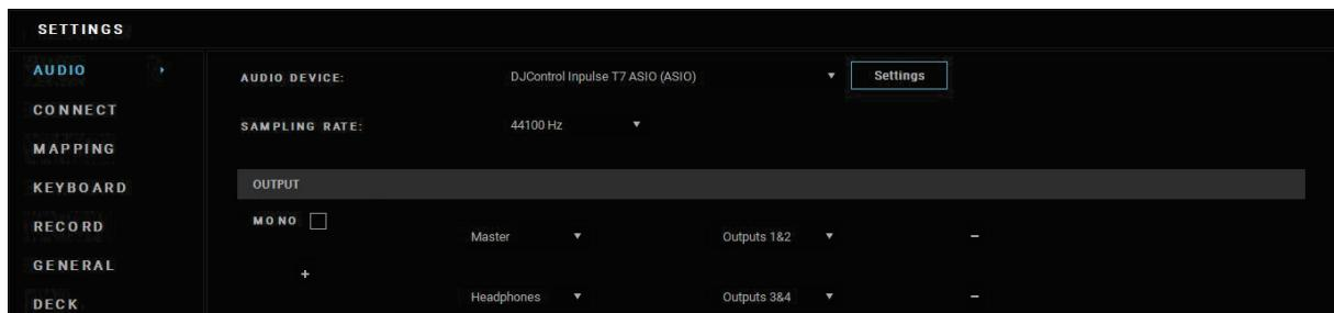
Once the software begins using the ASIO driver, the ASIO settings can no longer be modified in the control panel. This is perfectly normal, and indicates that the ASIO driver is in use.
