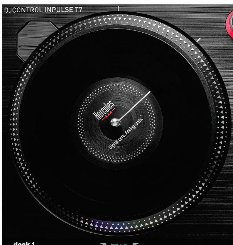
**Felt slipmat:** placed between the motorized platter and the vinyl record. It protects the vinyl record from rubbing against the platter, and reduces vibrations when playing the record.
