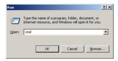
In the window that is displayed, enter the command "ipconfig" and then press the "Enter" key.
