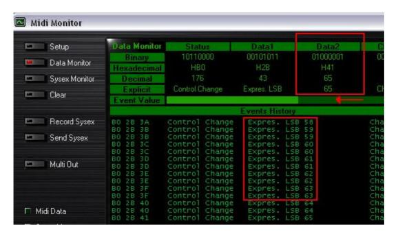
This test can also help determine if some of the controls of the DJ Control MP3 are not working correctly. For example, if the crossfader is only halfway to his course but already displays its maximum value of 127.
