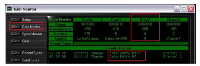
For knobs and sliders, who are incremental controls, you should normally get values **between 0 and 127**, depending on the position of the controller. The **Event Value** should also display the relative position of the control being used according to the value.
