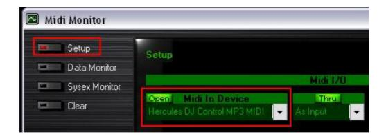
By default, the **MIDI In Device** should be **Open**. This is necessary for the software to be able to read the incoming data from the DJ Control.
