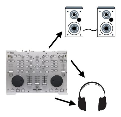
In order to connect regular computer speakers or a home sound system to **Output 1-2** on the back of the Rmx, a **RCA male to 3.5mm female adapter** may be required.
