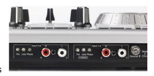
Note that when a microphone is used as input, Input 1-2 is not available.
