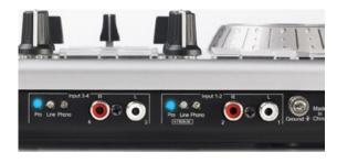
You can select between **Pro level (+4dBu)** and **Boosted level (+8dBu)**, depending on your device output level (Check the user manual for more details).
